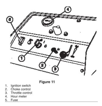
**Choke Control** (Fig. 6)—To start a cold engine, close the carburetor choke by pulling the choke control out to the ON position. After the engine starts, regulate the choke to keep the engine running smoothly. As soon as possible, open the choke by pushing it downward to the OFF position. A warm engine requires little or no choking.
