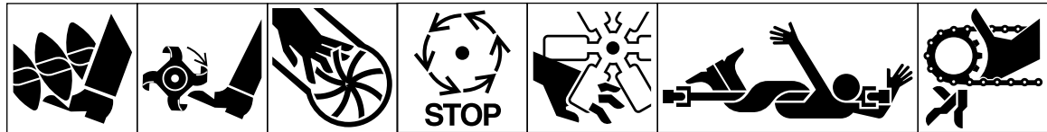
Cutting or entanglement of foot, rotating auger Severing of foot, rotating knives Severing of fingers or hand, impeller blade Wait until all machine components have completely stopped before touching them Severing of fingers or hand, engine fan Whole body entanglement, implement input drive line Fingers or hand entanglement, chain drive
