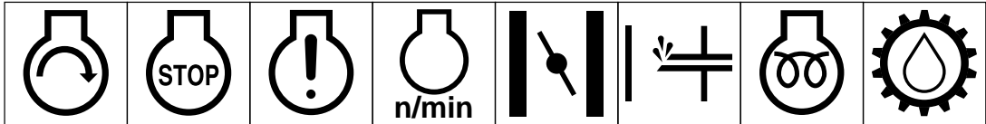
Engine start Engine stop Engine failure/malfunction Engine rotational speed/frequency Choke Primer (start aid) Electrical preheat (low temperature oil start aid) Transmission
