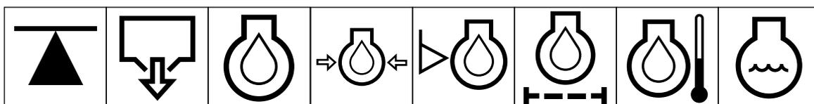
Jack or support point    Draining/emptying    Engine lubricating oil    Engine lubricating oil pressure    Engine lubricating oil level    Engine lubricating oil filter    Engine lubricating oil temperature    Engine coolant
