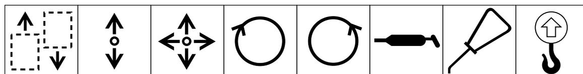
Machine travel direction, forward/rearward    Control lever operating direction, dual direction    Control lever operating direction, multiple direction    Clockwise rotation    Counter-clockwise rotation    Grease lubrication point    Oil lubrication point    Lift point
