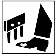
CRUSHING OR PUNCTURE OF FOOT, CORING HEAD
