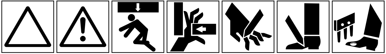
SAFETY ALERT SYMBOL GENERAL HAZARD SAFETY ALERT CRUSHING OF WHOLE BODY, APPLIED FROM ABOVE CRUSHING OF FINGERS OR HAND, FORCE APPLIED FROM SIDE CUTTING OF FINGERS OR HAND CUTTING OF FOOT CRUSHING OR PUNCTURE OF FOOT, CORING HEAD
