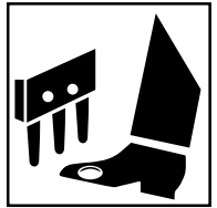
CRUSHING OR PUNCTURE OF FOOT, CORING HEAD
