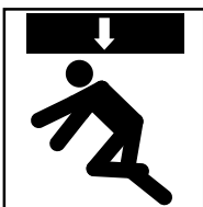
CRUSHING OF WHOLE BODY, APPLIED FROM ABOVE
