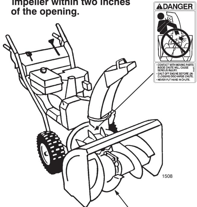
The low-speed auger has a moving pinch point close to the opening.
