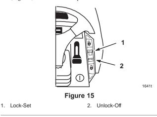
2. This locks the traction control in position and your foot can then be removed from the traction control. A constant ground speed will be maintained.
