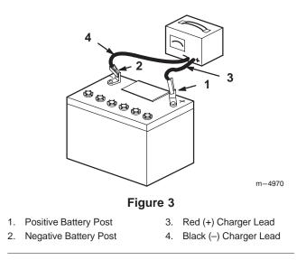
**9.** Install the battery in the tractor and connect the battery cables. Refer to the Installing the Battery on page 31.
