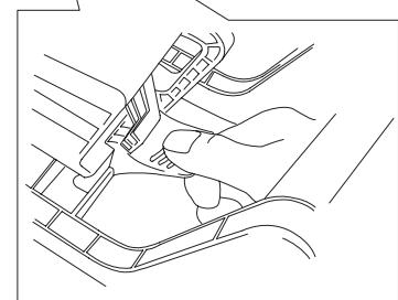
**Important:** The vacuum will not run unless the vacuum tube is locked in place.
