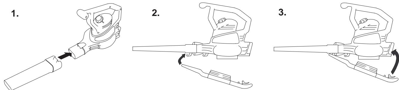
**Important:** You must install the blower tube before installing the inlet cover because the inlet cover hooks onto the blower tube. The blower will not run unless the bottom inlet cover is locked in place.
