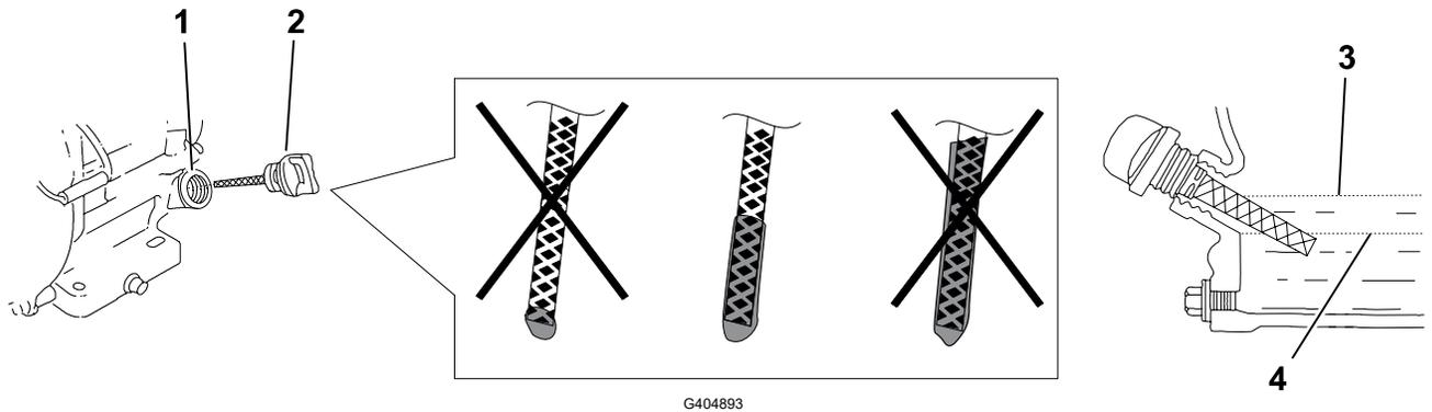
3. Remove the dipstick ② by rotating it counterclockwise.
