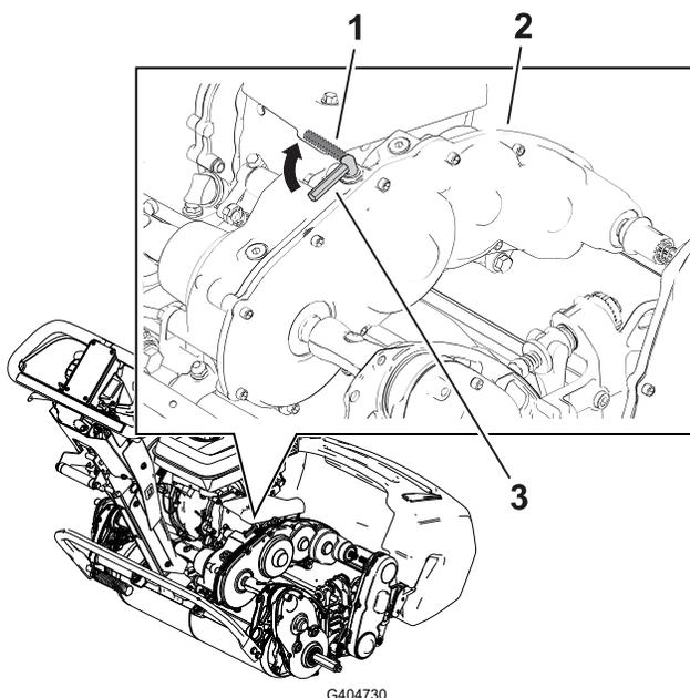
① Traction-engagement lever—DISENGAGED position
