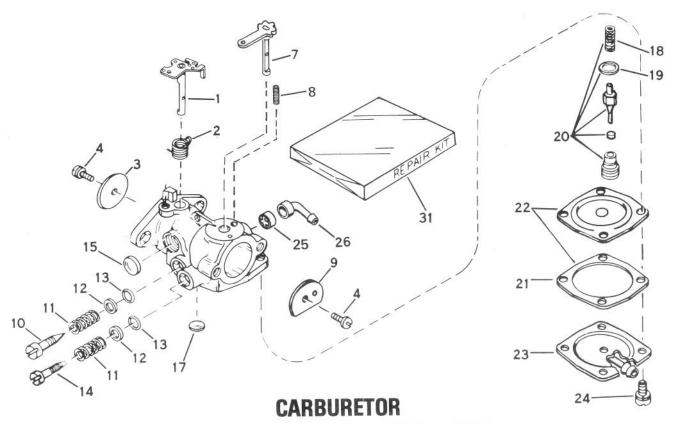
NO. 632103 — Engine Model AH520 Type 1584A NO. 632035 — Engine Model No. AH520, Type 1584B NO. 632141 — Engine Model No. AH520, Type 1601 & 1601A NO. 632165 — Engine Model No. AH520, Type 1601B
