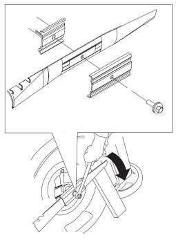
**2.** Remove the blade and save all blade mounting hardware.
