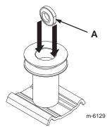
**2.** Install the blade driver onto the crankshaft without allowing the key to go into the slot in the crankshaft.
