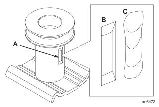
**Note:** The spacer in this kit is compatible only with the blade driver with a welded key (C). Contact an Authorized Service Dealer to purchase a new blade driver with a welded key.
