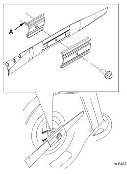
**6.** Inspect the blade driver key (A). If the key is stamped into the side (B) or if the key is damaged on the inside of the blade driver, install a new blade driver with a welded key (C).
