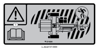
① Warning—read the *Operator's Manual*; keep away from the area shown while in operation.
