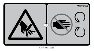
1 Cutting hazard—keep away from moving parts.
