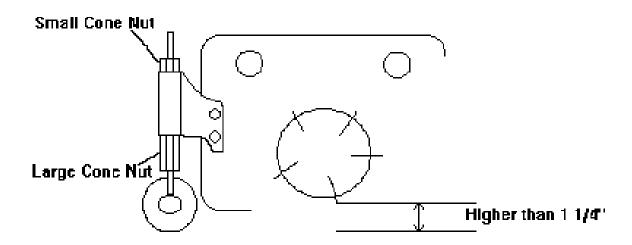
Use Large Cone Nut (92-9249) on bottom of Collar when H.O.C. is 1-1/4" (32 mm) or greater.
