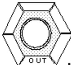
**"OUT" must be visible when installed**
