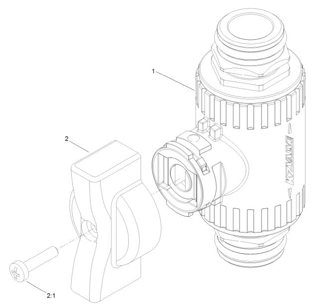
**Shutoff Bypass Valve Assembly No. 131-5838**
