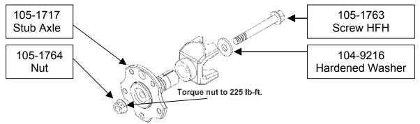
\* Caution: Many air impact wrenches do not exceed 100 ft.lbs.(136 Nm) torque capacity.
