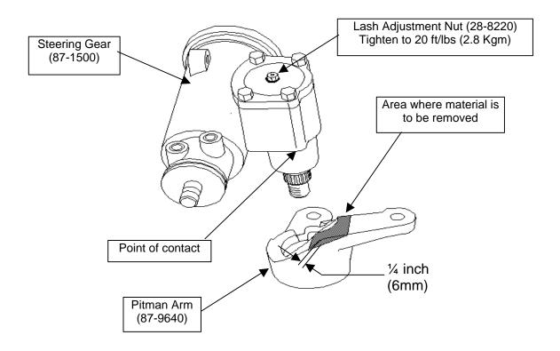
Note: Torque Retaining Nut to 180-210 ft-lbs (25-29 Kgm)
