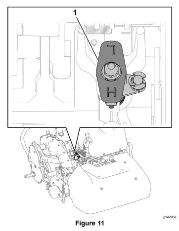
1. Reel-speed-control knob (shown in the high-reel-speed position)
