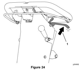
1. Apply force to release the parking brake.
