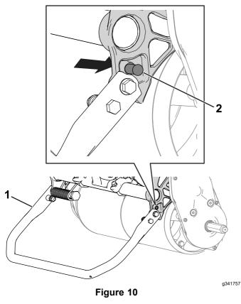
1. Kickstand—CUTTING-UNIT 2. Spring pin SERVICE position
