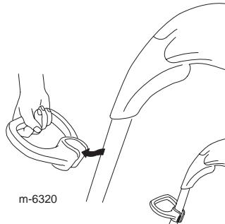
2. Install the guard as shown, snapping it into both sides of the trimmer.
