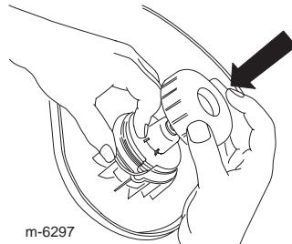
3. Twist the cap on securely clockwise.
