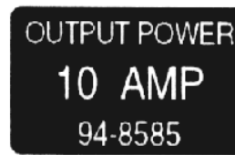
Part No. 94-8585; Located at the Aux. Fuse Block of Workman ® and MULTI PRO ® Sprayers
