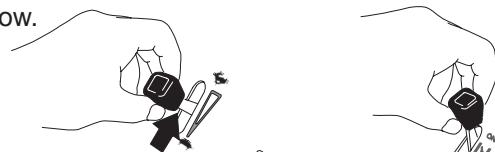
3. Turn the ignition key to Start until the engine starts.
