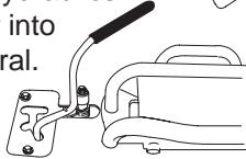
4. Pull back the collar on the female hydraulic couplers and pull the attachment couplers from the traction unit couplers.
