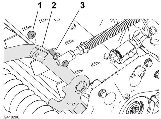
5. Align the studs ③ of the left hose guide with the holes in the cutting-unit frame and the turf-compensator bracket ①.
