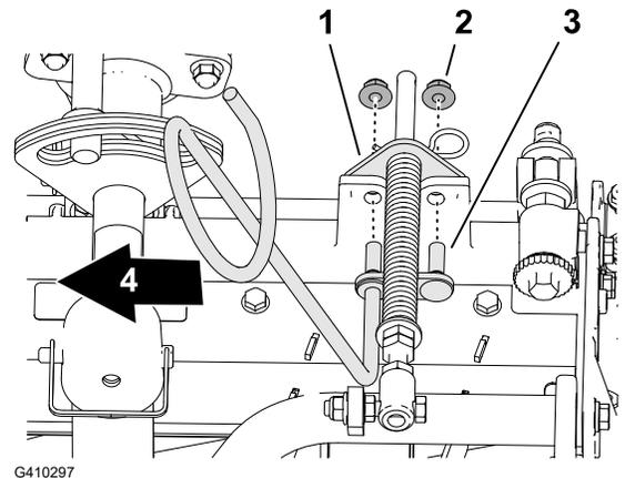
7. Torque the locknuts and bolts to **37 to 45 N·m (27 to 33 ft·lb)**.
