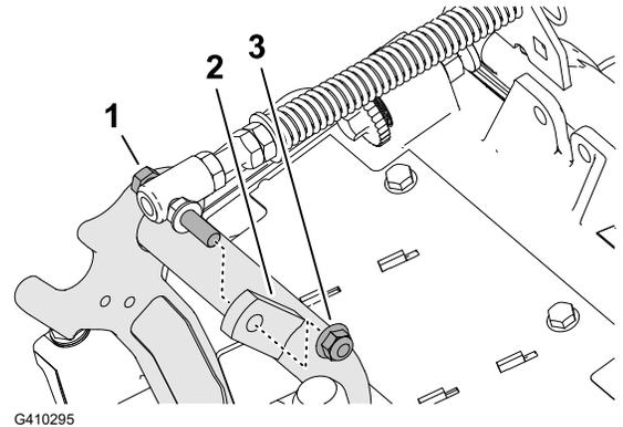
4. Assemble the bolt ③ of the turf compensation spring to the right tab ② of the carrier frame with the flange locknut (3/8 inch) ①.
