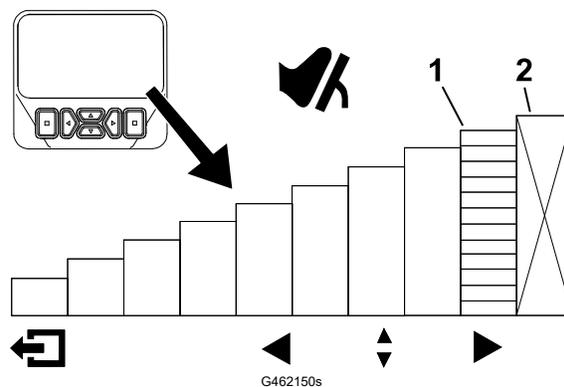
① Indicates the maximum traction speed (pedal stop)
