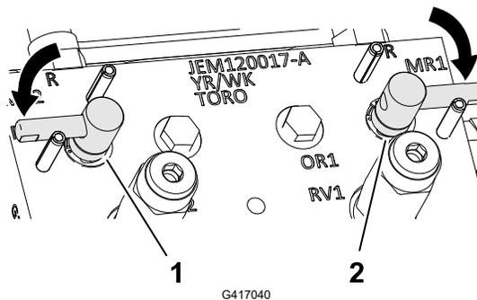
① Backlap lever (mow position—front cutting units)
