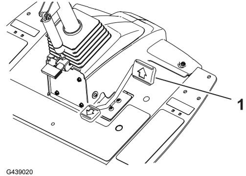
This traction system allows you to customize the acceleration settings for operator comfort and course conditions.
