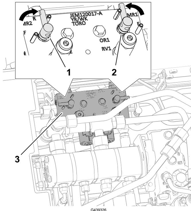
① Backlap lever (backlap position—front cutting units)
