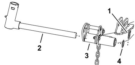
2. Assemble the pivot yoke (3) onto the carrier frame shaft (4).
