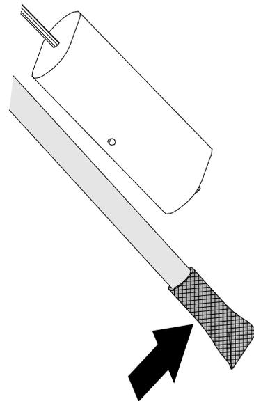
2. Carefully assemble the fuel pick-up tube and float into the fuel tank.
