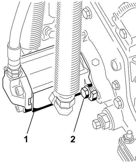
4. Rotate the motor counterclockwise until the flanges encircle the bolts, and then tighten the bolts.
