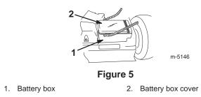
**Note:** Use a flat-head screw driver to unclip the battery cover (Fig. 6). Unclip both ends of the battery cover before removing it to prevent damaging it.
