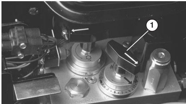
Figure 42 1. Reel speed control
