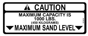
Part No. 87-0470: Located on rear of Hopper.
