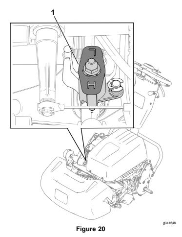
Reel-speed-control knob (shown in the high-reel-speed position)
