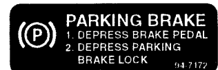
Part No. 94-7172: Located on left side of Dash Panel, under Steering Wheel.
