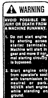
#87-0430 Located on left-hand side of Seat Support.
