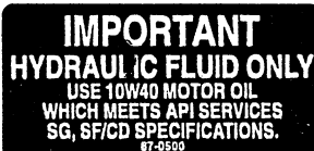
#87-0500 Located on top of Hydraulic Tank.
