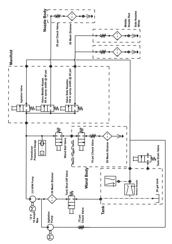
Sprayer System Schematic (Rev. A)
