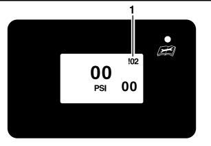
1. Fault code !02 (motor overcurrent)
