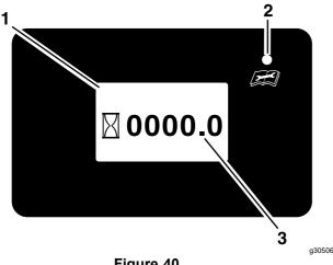
Figure 40 Engine Hours Screen
