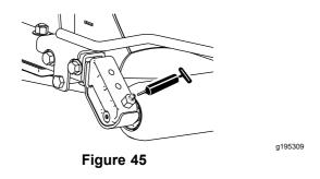
**Note:** Ensure that the grease groove in each roller mount aligns with the grease hole in each end of the roller shaft. To help align the groove and hole, there is also an alignment mark on an end of the roller shaft.
