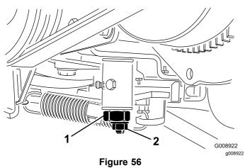
1. Traction adjustment cam 2. Locknut
