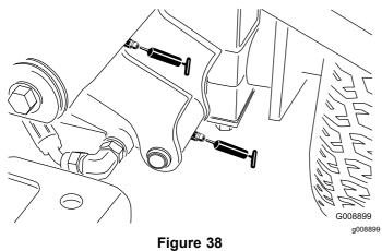
2 right, front lift-arm pivots and lift cylinder (Figure 39)
