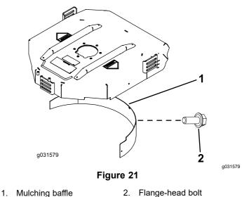
3. Verify that the mulching baffle does not interfere with the tip of the blade and does not protrude inside the surface of the rear chamber wall.
