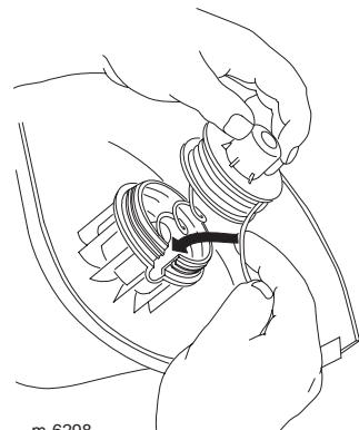
2. Holding the line and spool, place the cap over the spool.
