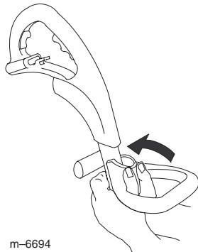
**Important:** Do not lay the trimmer down or against something while installing the assist handle. If you push on the trimmer shaft, it could break.
