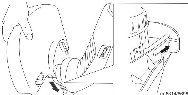
2. Snap the guard into place and secure the hooks under the guard on to the trimmer.
