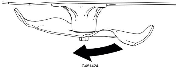
3. Measure from the tip of the blade to the level surface.
