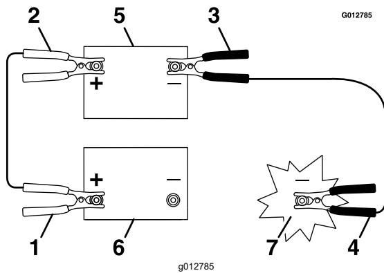
① Positive (+) cable on discharged battery
