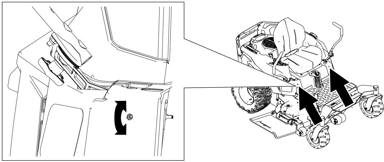
4. Rotate the bolt to decrease the speed for that particular wheel.
