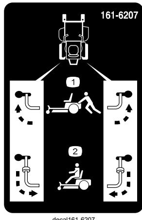
① Bypass lever position for pushing the machine
