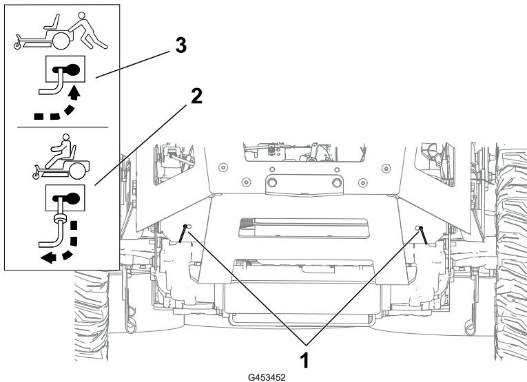
4. Move both bypass levers forward through the slotted hole and over to lock them in place
