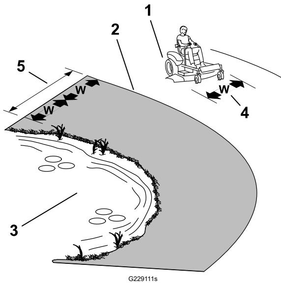
① Safe Zone—use the machine here on slopes less than 15° or flat areas.
