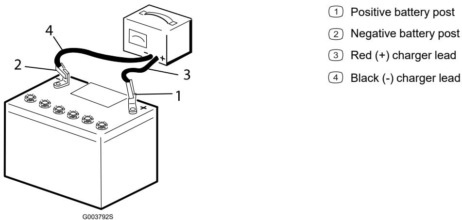
3. When the battery is fully charged, unplug the charger from the electrical outlet (if applicable), then disconnect the charger leads from the battery posts.
