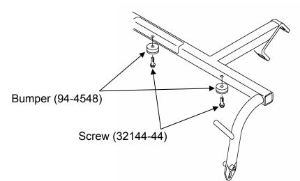
Remove Bumpers from Carrier Frames when installing Cutting Units other than Models 04610 or 04611.
