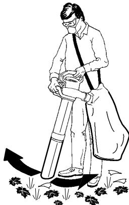
**Important:** Do not force the vacuum tube into a pile of debris or hold the tube upright while force feeding debris into the tube. Either action may clog and damage the impeller. If the vacuum starts to vibrate or make abnormal noise, stop it, **unplug** the cord, and check for the cause.
