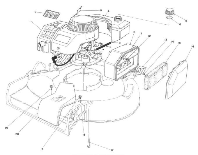
ENGINE ASSEMBLY (used on units with Serial No. 6000101-6004101)
