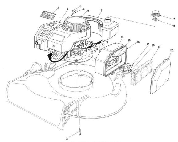
ENGINE ASSEMBLY (Model No. 47PF5) (used on units with Serial No. 7000001 - 7002104)
