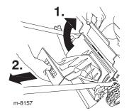
3. Route the starter rope around the lower rope guide.
