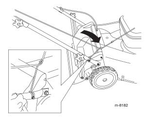
**Note:** The lower rope guide releases the starter rope when you pull the recoil start handle.
