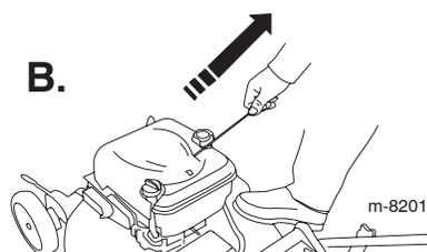
3. If the mower does not start in 1 or 2 pulls (or within 5 seconds using the electric starter), press the primer button 1 or 2 times and try starting it again.
