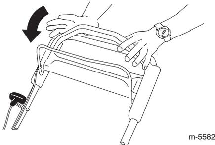
**Important:** When you release the blade control bar, the blade should stop within 3 seconds. If it does not stop properly, stop using your mower immediately and contact an Authorized Service Dealer.
