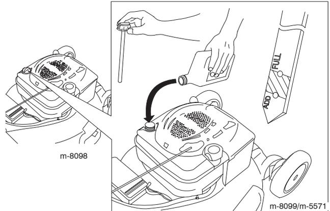
2. **Slowly** pour oil into the oil fill tube until the oil level reaches the **Full** line on the dipstick. **Do not overfill.** (Max. fill: 20 oz., type: SAE 30W detergent oil with an API service classification of SF, SG, SH, SJ, SL, or higher.)
