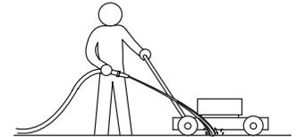
The water will splash into the path of the blade, cleaning out the clippings.
