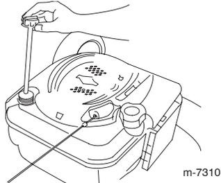
2. Tip the mower onto its side (with the air filter up) to drain the used oil out through the oil fill tube.
