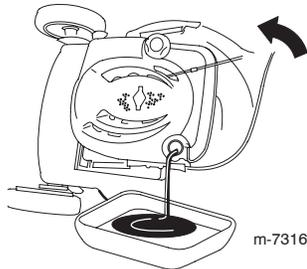
3. **Slowly** pour oil into the oil fill tube until the oil level reaches the **Full** line on the dipstick. **Do not overfill.** (Max. fill: 20 oz., type: SAE 30W detergent oil with an API service classification of SF, SG, SH, SJ, SL, or higher.)
