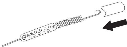
7. Hook the cable spring into the **bottom** hole of the control bar.
