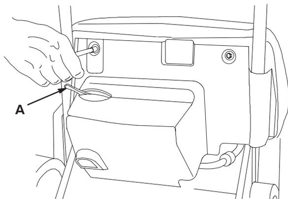
2. Pull the top of the shroud to the rear until the choke lever (A above) clears the slot.
