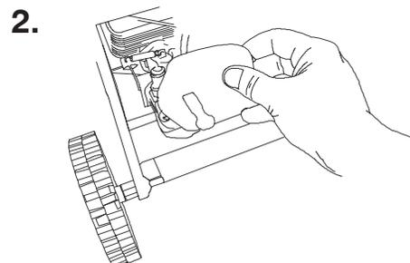
2. As you install the new lower shroud onto the snowthrower, guide the choke lever through the slot.
