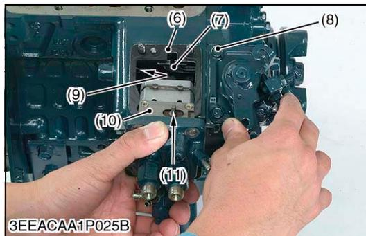
**Injection Pump, Fuel Feed Pump and Speed Control Plate
