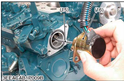
**Injection Pump, Fuel Feed Pump and Speed Control Plate (for Energize to Run Type Engine Stop Solenoid) (Continued) (When reassembling)**
