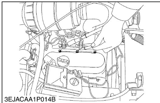
**Glow Plug Lead Terminal Voltage**
