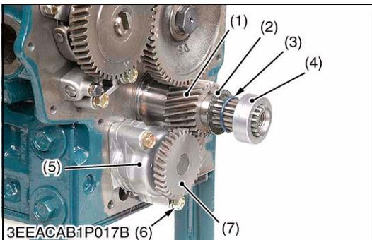
**Oil Pump and Crankshaft Gear (One-side Maintenance Type)**
