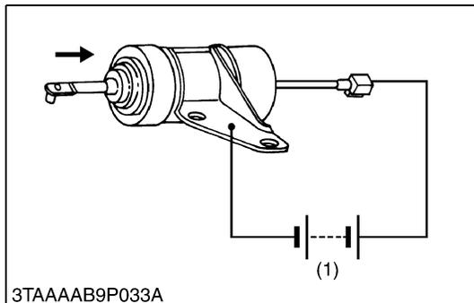
**Engine Stop Solenoid Test (Energize to Stop Type)**
