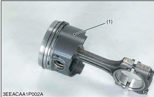
Piston's skirt is coated with **molybdenum disulfide**★, which reduces the piston slap noise and thus the entire operating noise.
