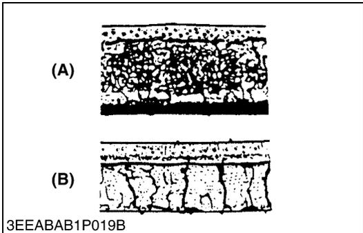
**Fan Belt Damage and Wear**
