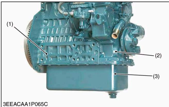
The oil pan is extended under the gear case. Therefore, the height of the engine can be lowered more than so far while securing a necessary amount of oil.
