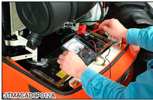
**Alternator on Unit Test**
