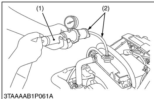
**Radiator Water Leakage**
