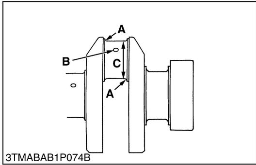
**Oil Clearance between Crankpin and Crankpin Bearing**
