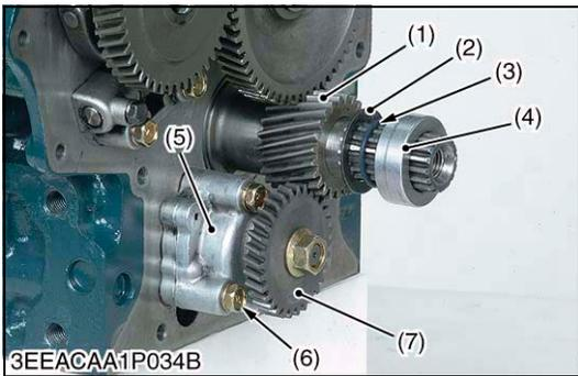
**Oil Pump and Crankshaft Gear**
