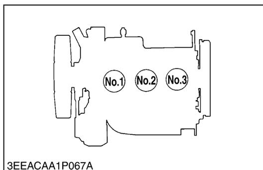
The cylinder numbers of KUBOTA diesel engine are designated as shown in the figure.
