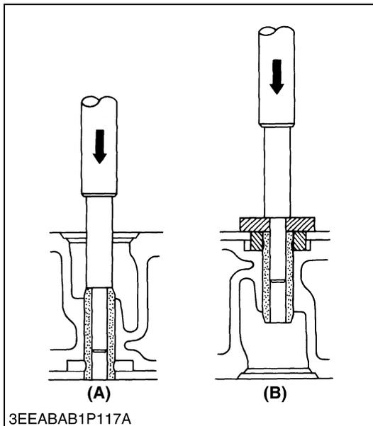
**Replacing Valve Guide**
