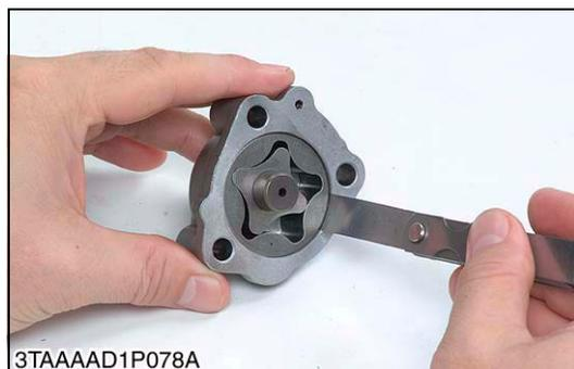
**Clearance between Outer Rotor and Pump Body**
