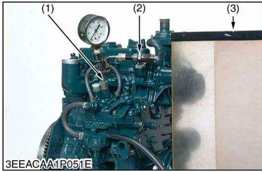
**Fuel Tightness of Pump Element**
