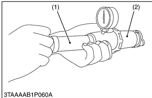
**Radiator Cap Air Leakage**
