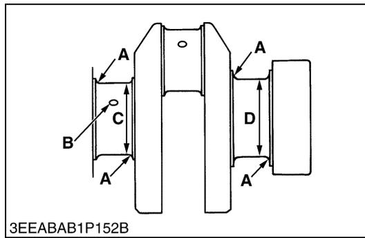
**Oil Clearance between Crankshaft Journal and Crankshaft Bearing 2 and Crankshaft Bearing 3 (Continued)**
