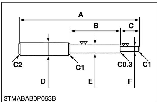
**Valve Guide Replacing Tool**
