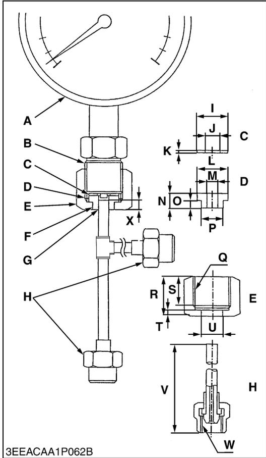
**Injection Pump Pressure Tester**
