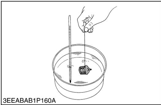
**Thermostat Valve Opening Temperature**
