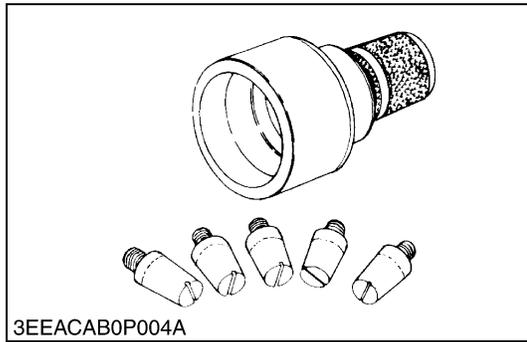
**Crank Sleeve Setter (for Z482/D662/D722/D782-E2B)**
