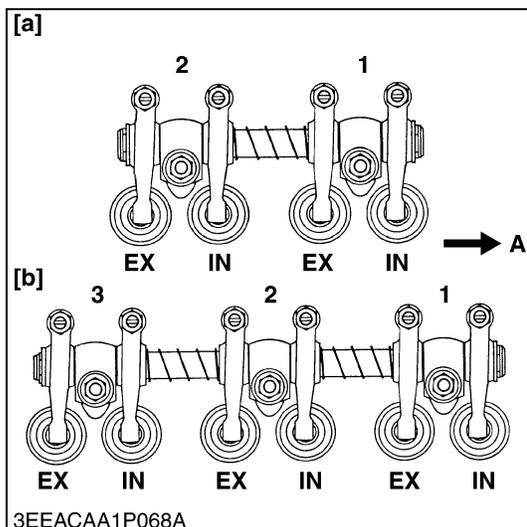
**Checking Valve Clearance**
