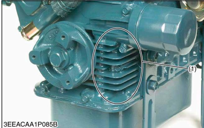
The cooling fin is set up around the oil passage in the gear case.
