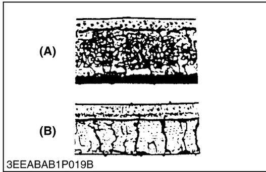
**Fan Belt Damage and Wear**
