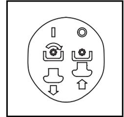
**NOTE:** The PTO knob **must** be in the disengaged (Blade Stop) position when starting the engine.
