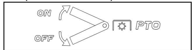
On models equipped with a manual PTO, the PTO lever is located on the left side of the dashboard next to the steering wheel. Move the PTO lever forward to engage the power to the cutting deck or other (separately available) attachments; move the PTO lever rearward to disengage the power.
