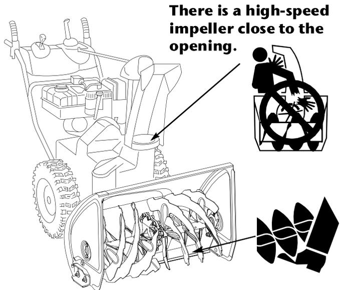
**There is a high-speed impeller close to the opening.**
