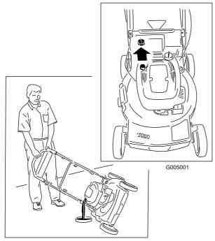
Slowly pour oil into the oil fill tube until the oil level reaches the Full line on the dipstick (Figure 23). Do not overfill. (Max. fill: 20 oz., type: SAE 30W detergent oil with an API service classification of SF, SG, SH, SJ, SL, or higher.)
