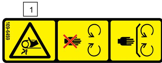
1. Entanglement hazard, belt – do not open or remove safety shields while engine is running, keep shields in place.
