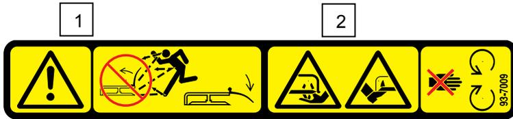
1. Warning – do not operate the mower with the discharge deflector up or removed; keep the discharge deflector in place.
