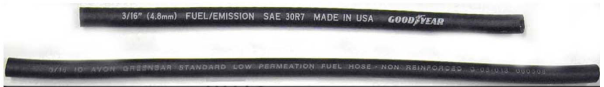
Figure 1 - (Top) 2005 and earlier standard fuel line/house, (Bottom) 2006 and later “Low Permeation” Hose.
