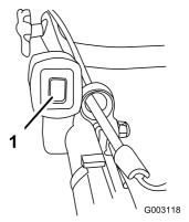
**Figure 21**1. Ignition toggle switch
